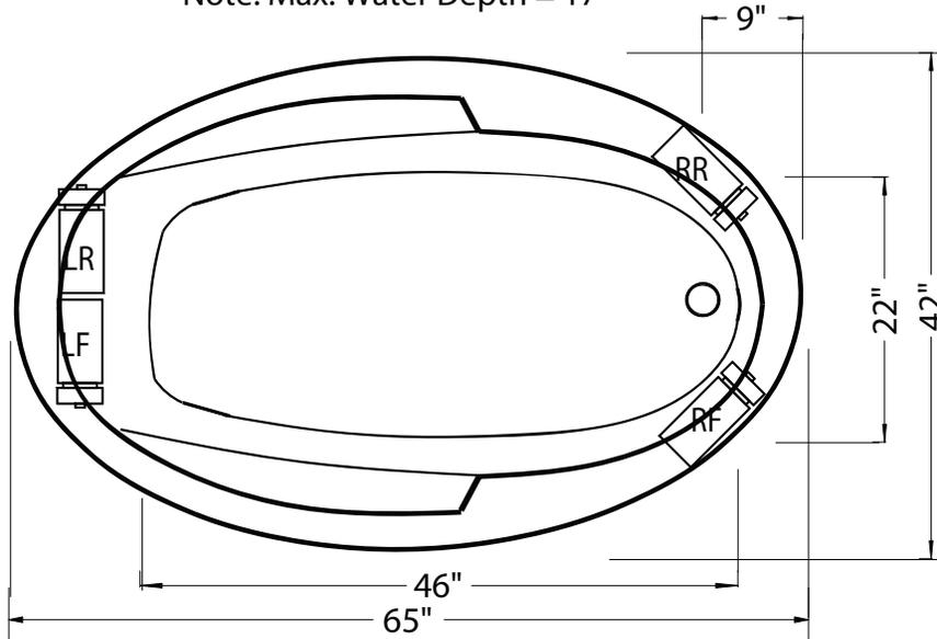
LF = Left Front Pump Location    RF = Right Front Pump Location
